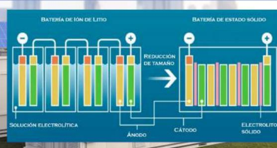
With the solid Electrolyte, a Reduction in the Size and Weight of the battery is achieved, maintaining the same power and an increase in autonomy, oxidation between anode and cathode is also avoided, increasing the life cycle as well as all the previously mentioned improvements.
